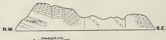
Figure 3. Cross section of southern slope of Big Limestone along B. B. (See map). The white areas indicate talus covered slopes. Vertical scale X 2.
